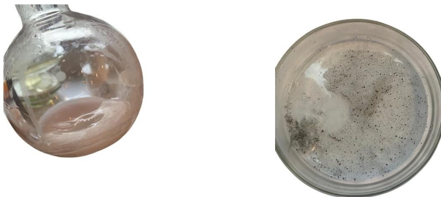
Fig. 2. A mixture of starch hydrogel with added graphene oxide
