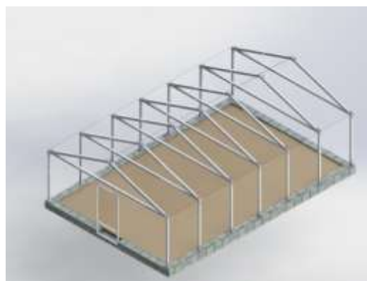
Fig. 1. Isometric of greenhouse frame
