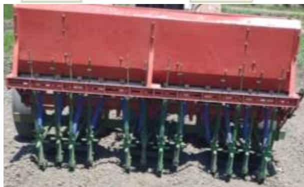
Fig. 1 and Photo 2. Side view and Elev. of the modified hill drill Source: Authors' own illustration.
