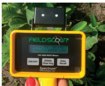
Figure 1. NDVI measuring device (source: Original photo, Sorina Nițu)
