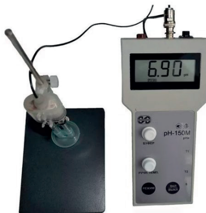
Figure 3. Portable millivoltmeter pH-150
