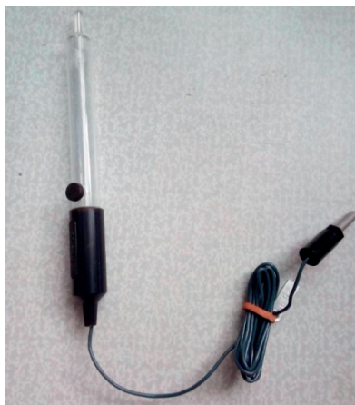
Figure 2. Auxiliary silver chloride electrode EVL-1M
