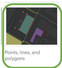
Figure 4: the three built in attributes for capture and their representation on a map. Points (with camera option), Lines (with tracing option) and polygons (tracing option).
