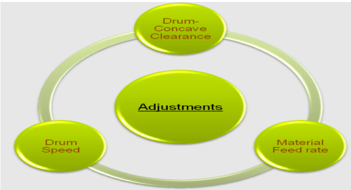
Fig. 2. Machine parameters that affect threshing and separation losses.
