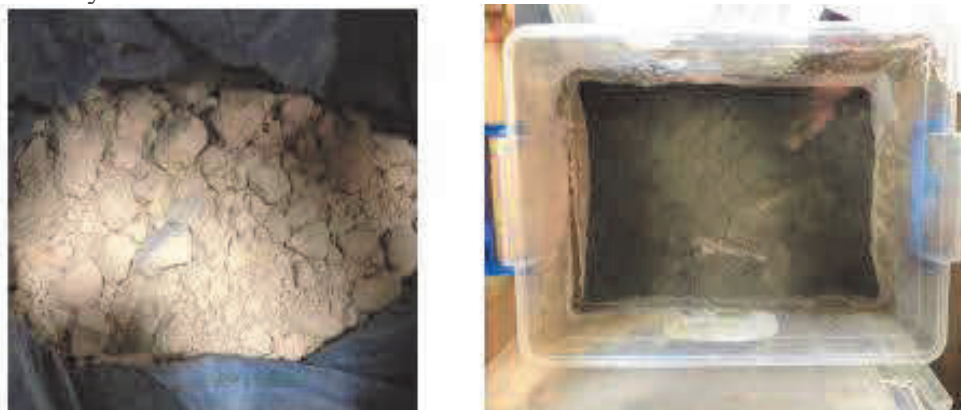
Figure 1. Burned filter sludge (left side) and unburned filter sludge (right side)
