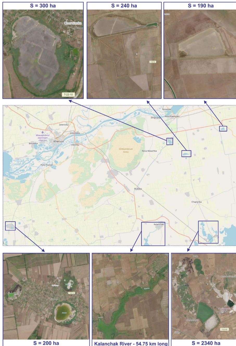
Fig. 8 Drainage of waterbodies in the temporarily occupied territory on the left bank of Kherson as of 2024, according to the Sentinel 2 L2 data
