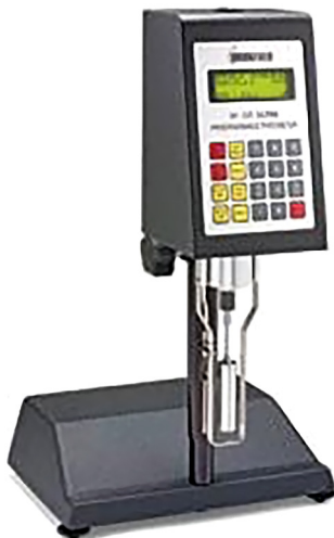
Fig. 2.11 Brookfield DV-III viscometer
