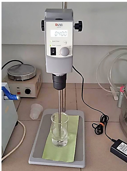
Fig. 2.10 Mixer for preparing a homogeneous hydrogel solution
