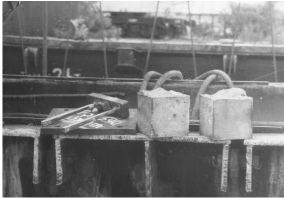
Figure 4.22. Compressed cube samples and wedge device
