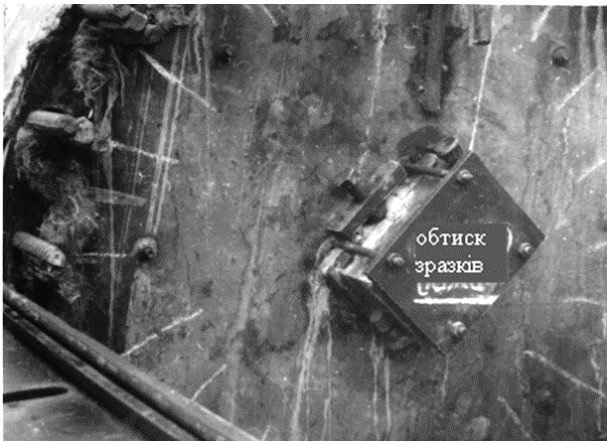
Figure 4.20. End of the pressure mold with a device for sampling concrete of standard sizes
