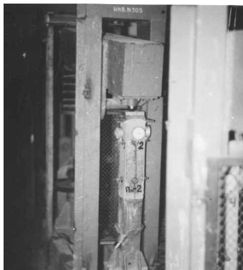
Figure 3.1 General appearance of the specimens compressed by the 'During-tensioning' method in a lever force device: a – specimen in the mold; b – specimen after removal from the mold without unloading
