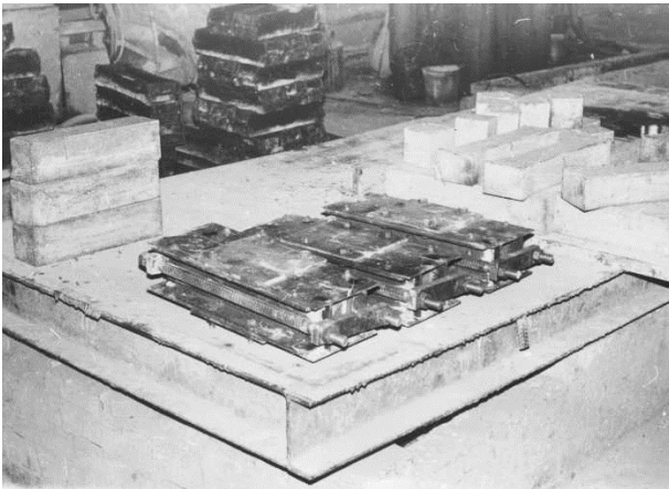
Figure 4.19. General view. Pressure mold for manufacturing compressed samples
