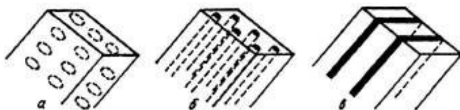
Fig. 19. Structural scheme of composite materials: a – dispersion-reinforced; b – fibrous; c – layered
