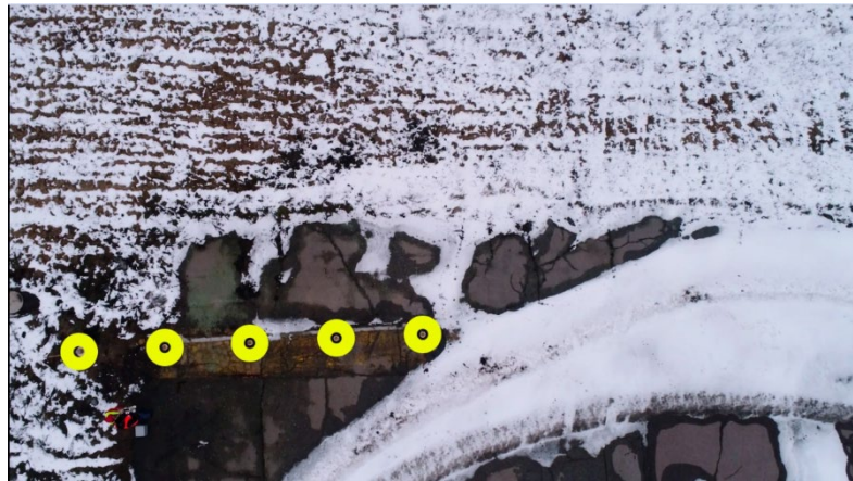
Fig. 1. Image of threshold lights of Kirovograd airfield runway with yellow colored overlays
