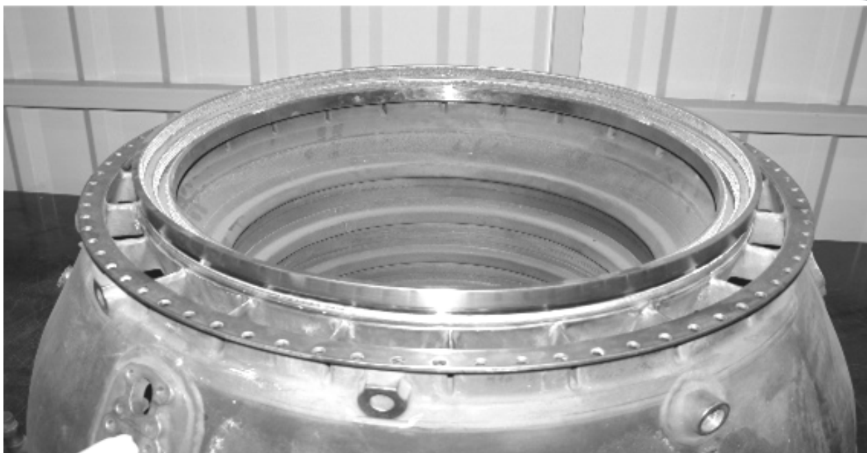
Figure 7 – Cracks in the body of the main combustion chamber
