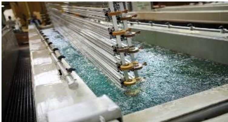
Fig. 1. Galvanic bath for coating
