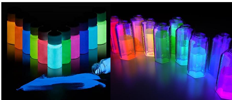
Fig. 2. An example of the glow of multicolored phosphors in the dark
