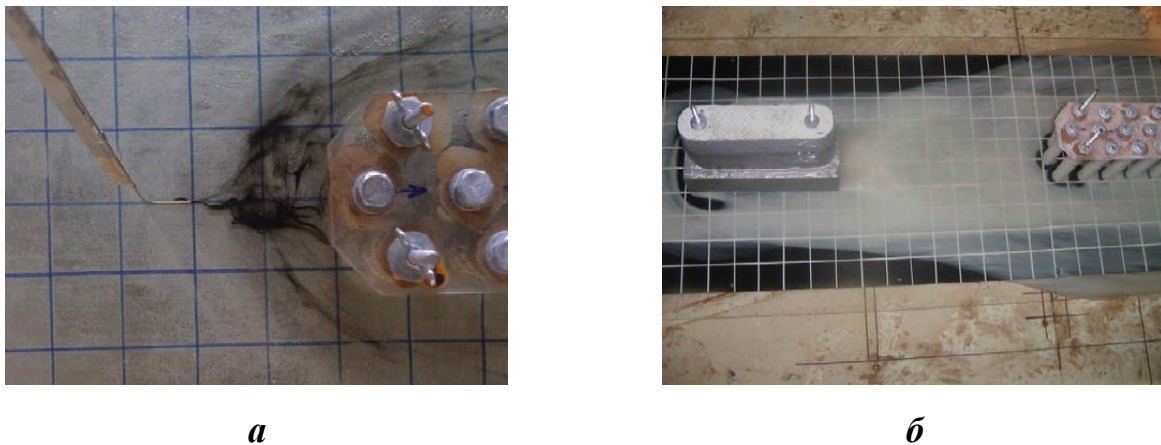
Fig. 1. Flow visualization around the pile models with the help of dyes (a) and a contrast coating that is washed away by water (b).
