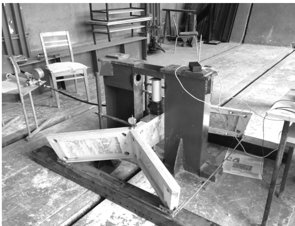
Fig. 1. A fragment of the dome under load
