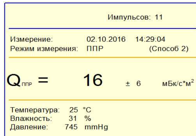
Fig. 4. Values of the meter when measuring RFD in soil near "Avanhard" stadium
