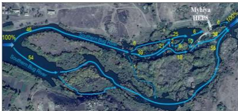
Fig. 5. Distribution of flow over the Southern Bug River water system in the region of Myhiya village in the low water period of the year. Figures on the diagram – the share of flow on a separate site in% of the total river flow (water consumption 43 \text{ m}^3/\text{s} ). According to the materials of full-scale shooting 18.07.2017
