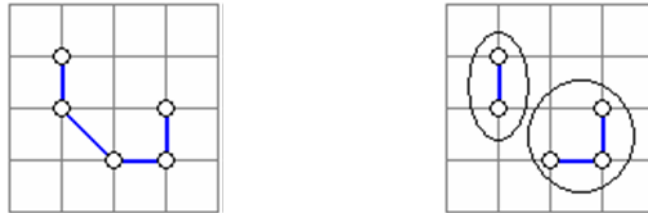
Pic. 3. Minimum spanning tree and two clusters formed after removal of longest rib. [5]
