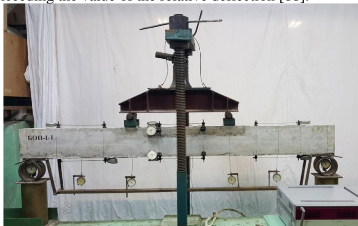
Photo 1. General view of the BOP-I-1 investigated beam at the test stand
