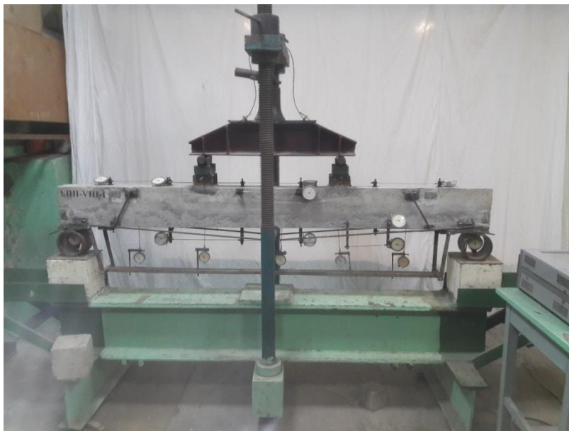
Photo 3. General view of the investigated beam at the test stand
