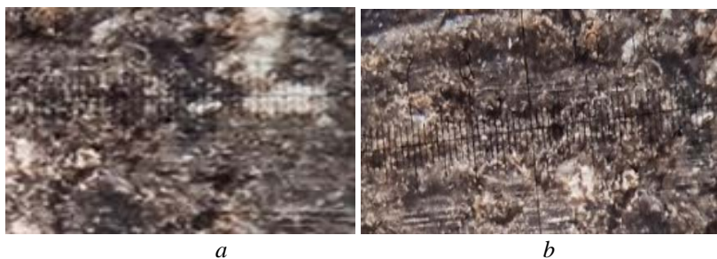
Fig. 3. Character of the surface structure of pellets and the density of gaps between the particles of raw material after pressing: a – outer surface of the SS-1 sample with a final pressure of 130.5 MPa; b – the same with a final pressure of 217.5 MPa
